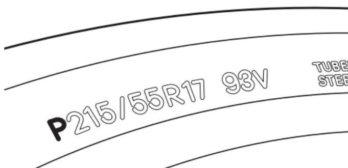
The maximum load capacity stamped on the sidewall of a P-metric tire is reduced by a factor of 1.1 when used on a light truck, a sport utility vehicle, or a trailer.
